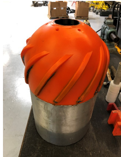
WWT JetReam, showing reamer blades surrounding jetting nozzles. Centerline nozzle opens when needed.
