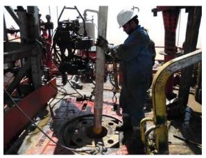
Photo showing the FLX-450 being run through the rotary table.
