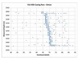
Hookload chart from the casing run. Notice the smooth trend, with no drag as the casing and shoe ran through the window at 3050m MD.
