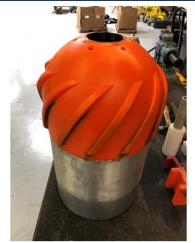
WWT JetReam, showing reamer blades surrounding jetting nozzles. Centerline nozzle opens when needed.
