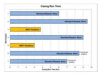
Chart comparing casing run times with and without the WWT FlexShoe.
