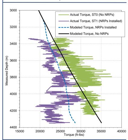
In addition to the torque reduction experienced, the casing was also protected due to the NRPs' ability to eliminate tool joint contact. Side-loads greater than 6,000 lbs/joint were modeled, which creates a high potential for casing wear. The increased risk of wear, due to the additional rotating hours for the sidetrack, was greatly reduced using NRPs.
