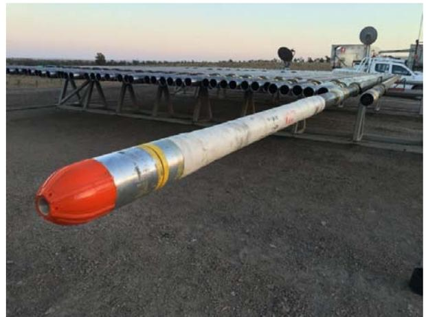
Photo showing WWT FLX-550 with JetGuide before being moved to the catwalk and lifted to the rig floor with the automated pipe handling system.
