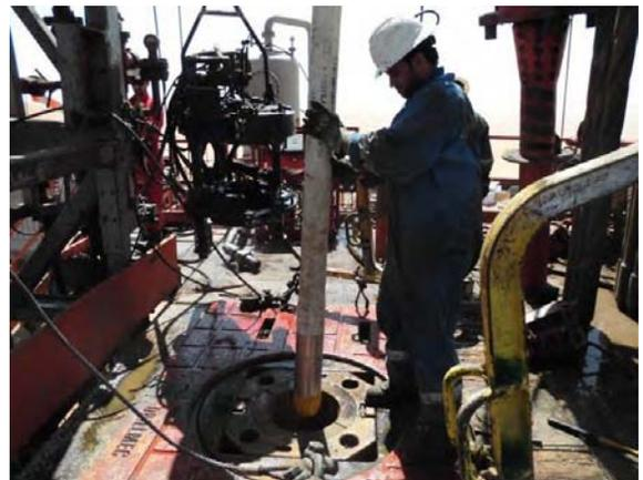
Photo showing the FLX-450 being run through the rotary table.
