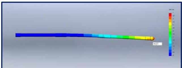
*Image of FEA analysis showing approximately 6" downward deflection in a horizontal wellbore. This allows the shoe to locate and enter a low-side sidetrack regardless of casing orientation.*
