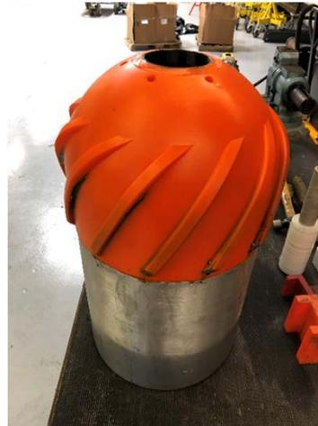
**WWT JetReam, showing reamer blades surrounding jetting nozzles. Centerline nozzle opens when needed.**
