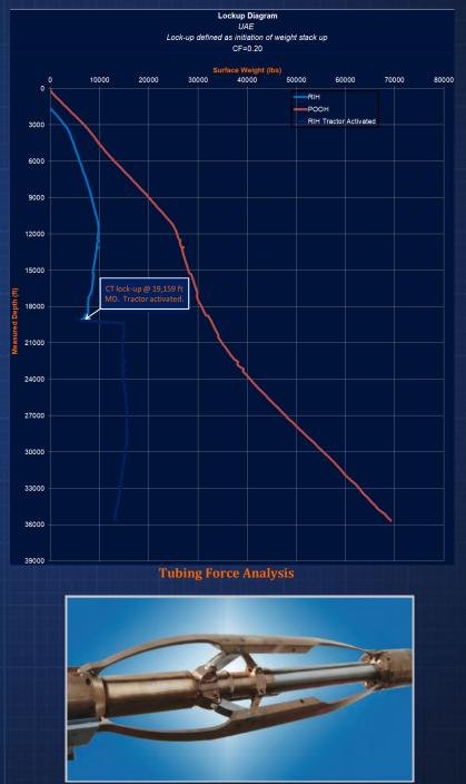
WWT Expandable Ramp Gripper Assembly
