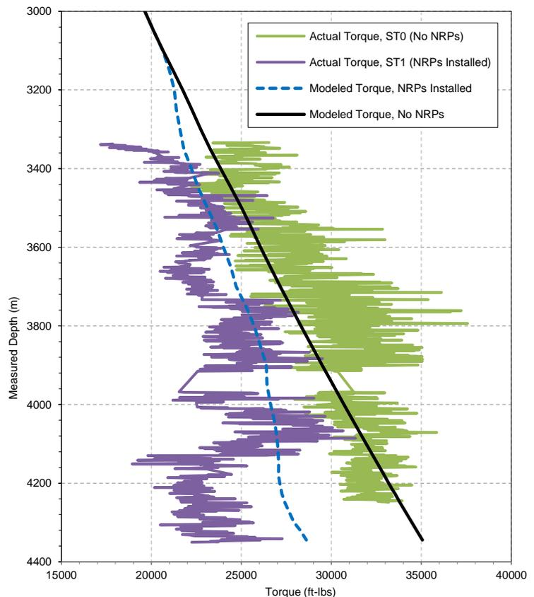
In addition to the torque reduction experienced, the casing was also protected due to the NRPs' ability to eliminate tool joint contact. Side-loads greater than 6,000 lbs/joint were modeled, which creates a high potential for casing wear. The increased risk of wear, due to the additional rotating hours for the sidetrack, was greatly reduced through the use of NRPs.
