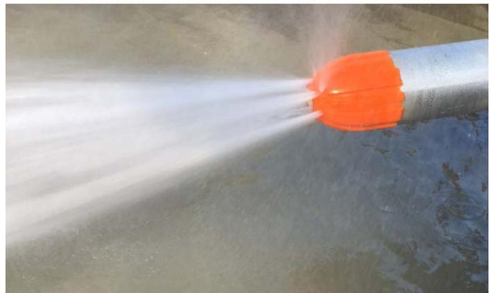
Photo showing the JetGuide high velocity flow at 150gpm. This was used to quickly wash though fill at the bottom of the hole.
