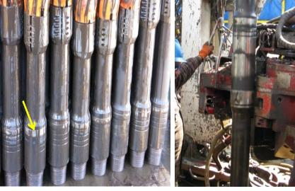
Figure 2: Tool joints with NRPs had visibly less wear, indicating stand-off was properly maintained.
