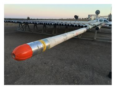
Photo showing WWT FLX-550 with JetGuide before being moved to the catwalk and lifted to the rig floor with the automated pipe handling system.
