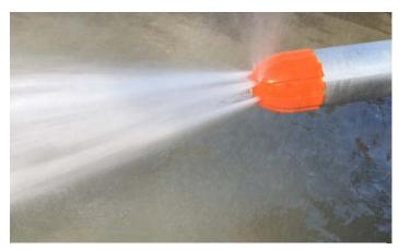
Photo showing the JetGuide high velocity flow at 150gpm. This was used to quickly wash though fill at the bottom of the hole.
