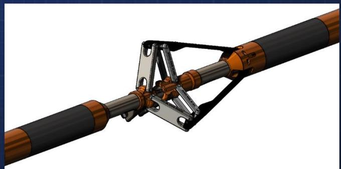
Figure 2 WWT Extreme Expansion Gripper assembly
